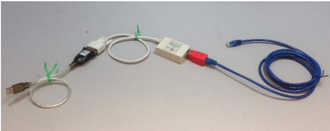
Figure 13- Cable Configuration for Direct Computer Connection
