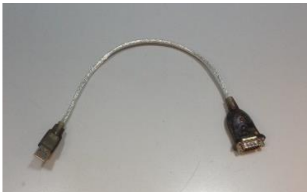
Figure 11- RS-232 to USB converter for connection via USB port
