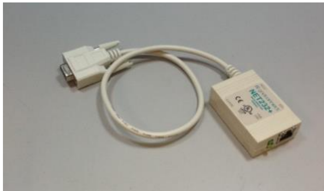
Figure 10- Ethernet to RS-232 converter for Connection via Serial port
