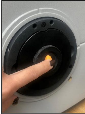
Holding Sample in Place
