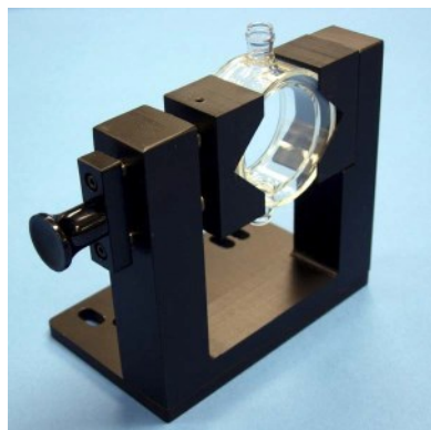
Flow Cell in Flow Through Cell Holder (D02-1009-960
